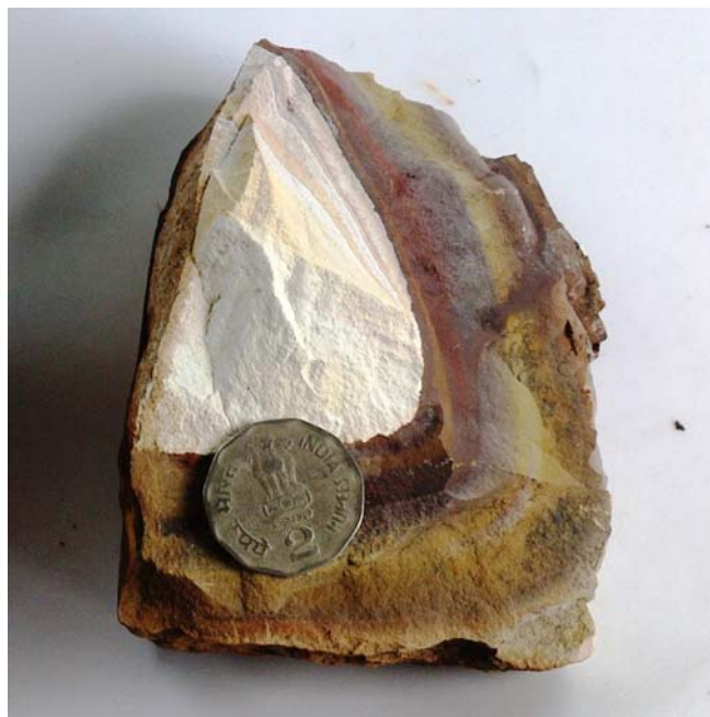
Fig. 4b: The cavity of the box work structure initially occupied by tuffaceous material of porcellanite converted to clay.
