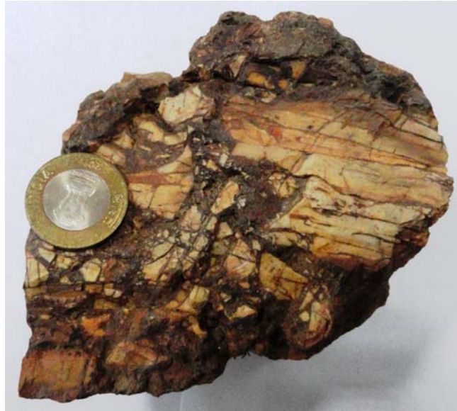
Fig. 4a: Brecciated porcellanite shale. Notice angular fragments of tuffaceous material.
